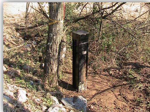
Typical Monitoring Well
